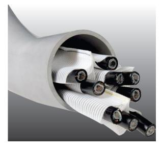
OptiCell™ innerduct is a flexible fabric system designed specifically for increasing conduit capacity. The unique textile construction allows OptiCell™ innerduct to conform to the shape of cables placed within, greatly reducing wasted space and increasing cable deployment efficiency.
